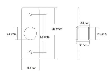
The CL-NT40 is a slimline request to exit device that uses infrared technology to grant access without needing to be touched.
